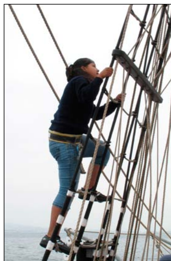
The ratlines are the only way to the yards and the topsails.
